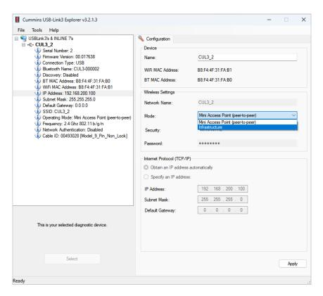
Figure 3.21 Wireless Settings: Mode Drop-down Menu
