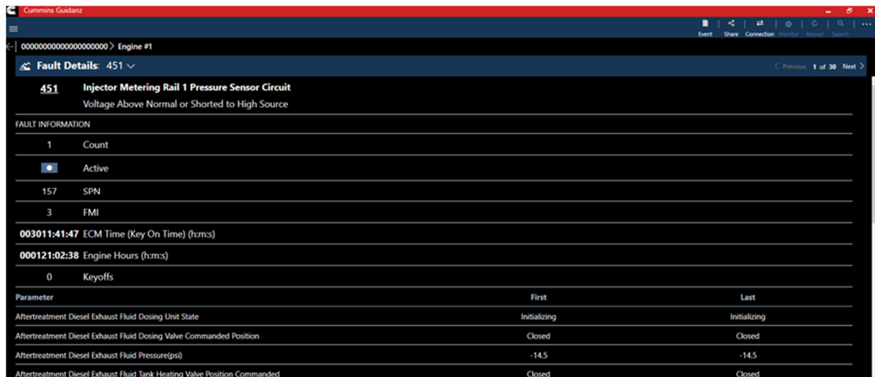
Figure 0-12 Cummins Fault Details and Snapshot
