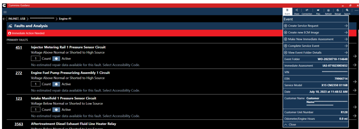
Figure 0-40 Create Service Request from Immediate Assessment
