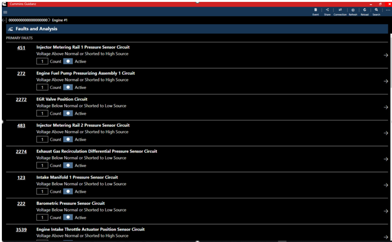
Figure 0-9 Faults screen from Cummins ECM
